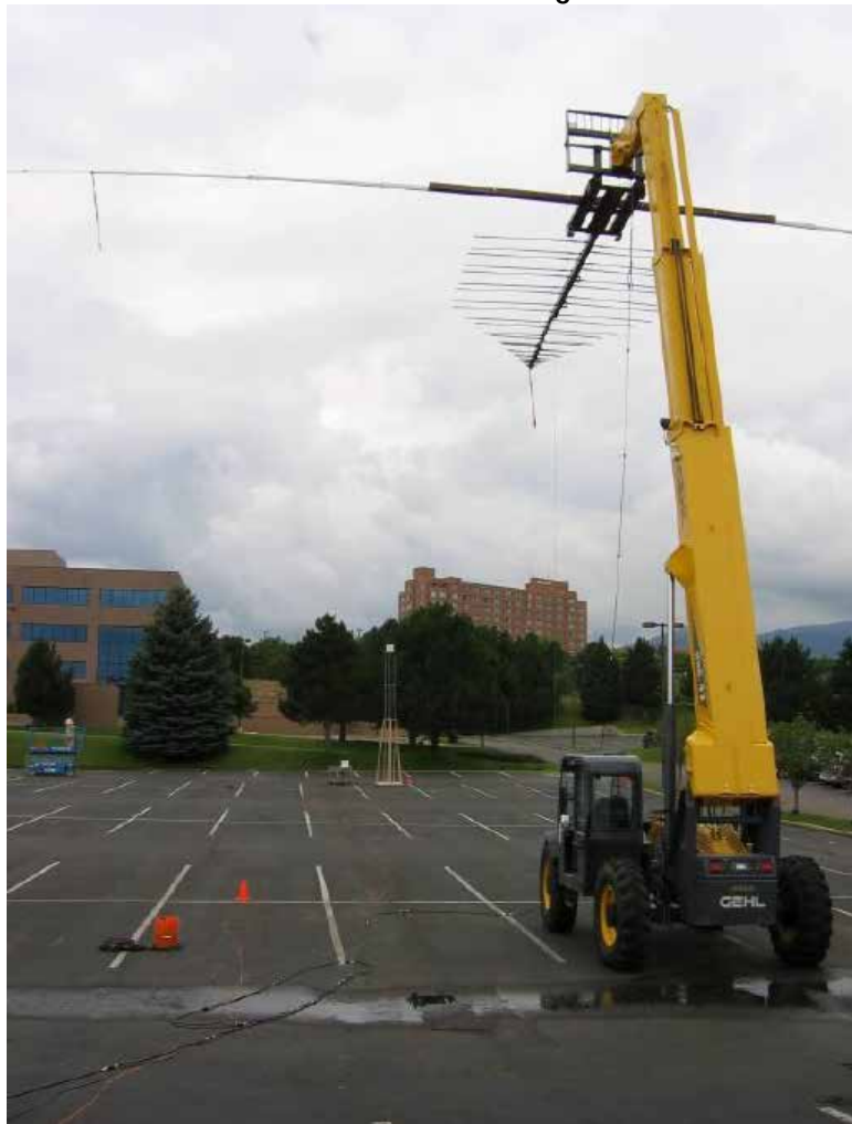
Figure 2 Proposed CWI Antenna System Mounting Scheme (Telehandler Height Maximum 55ft.)
