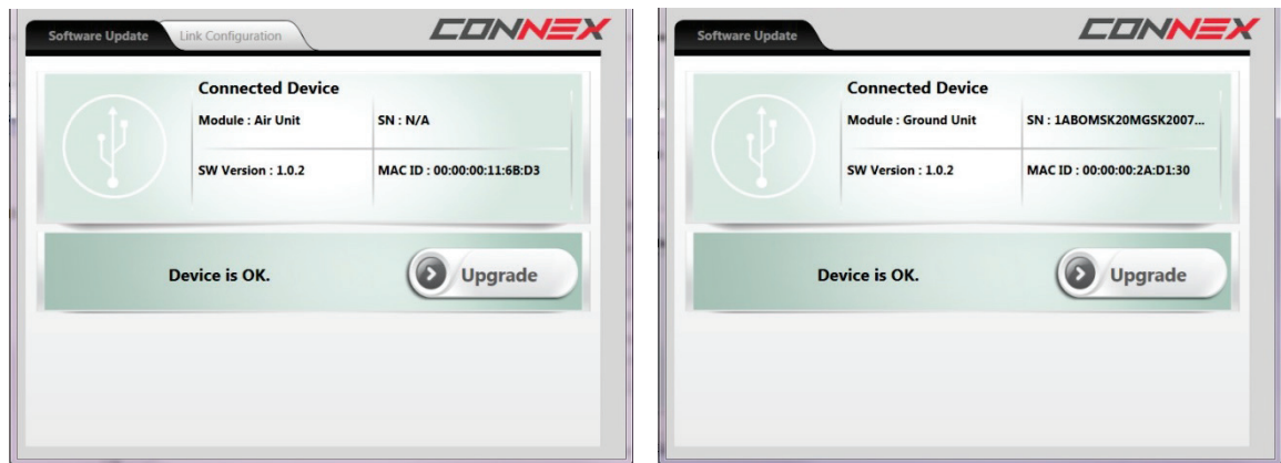
Figure 38: Upgrading the Air Unit (shown on left) or Ground Unit (shown on right)
