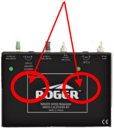
Location of Radiating antennas
