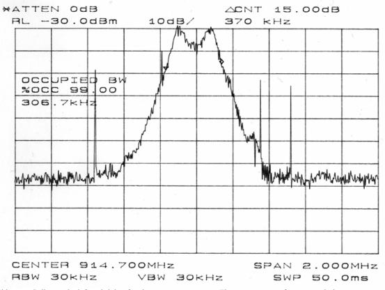
Sidenote: Spikes to the left and right of main spectrum are spurs. They are not part of our transmission spectrum.
