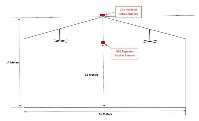
The radiating antenna is suspended 15 meters above the ground in the center of the hangar. The nearest wall is 27 meters away (54/2). In order to comply with NTIA regulations, the received signal power must be less than -140 dBm at a range of 57 meters from emissive antenna. Please note that emissive antenna is aiming down at the floor of the hangar.
