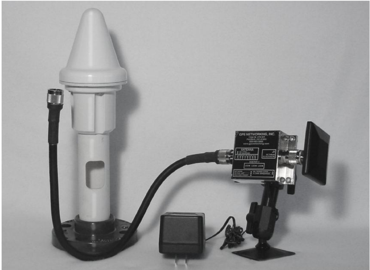
Figure 2 – Diagram of GPS Re-Radiation System
