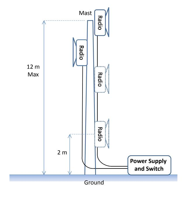
Figure 1 - Possible Radio Deployments on Mast
