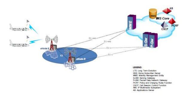
As a result of this trial, data services can be provided to airline passengers at higher rates and quality than available today. The radio technology used to provide the air-to-ground connectivity is new to this application. Additionally the WCS frequencies have not been previously used in such an application.
