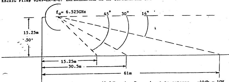
Tower mounted Andrew UHX 10-59D antenna; 43.2db gain. Power input to antenna = +40db = 10W.
