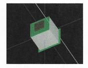
Except the antenna, TRSI satellites do not have deployable structures. For the orbital lifetime analysis, we had to calculate the cross section first. The software helps by providing the calculations based on a 3D model as input. The cross-section estimation is 4800 mm2. Input parameters and results of the cross-section calculations can be found in the supporting files for DRAMA/CROC outputs.
