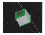
Except the antenna, MyRadar satellites do not have deployable structures. For the orbital lifetime analysis, we had to calculate the cross section first. The software helps by providing the calculations based on a 3D model as input. The cross-section estimation is 4800 mm2. Input parameters and results of the cross-section calculations can be found in the supporting files for DRAMA/CROC outputs.
