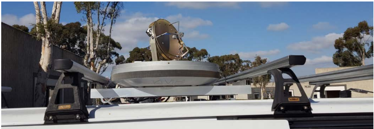
Figure 2 – Gogo K3 mobile test configuration. Antenna will be mounted to roof of van. Electronics and control inside.
