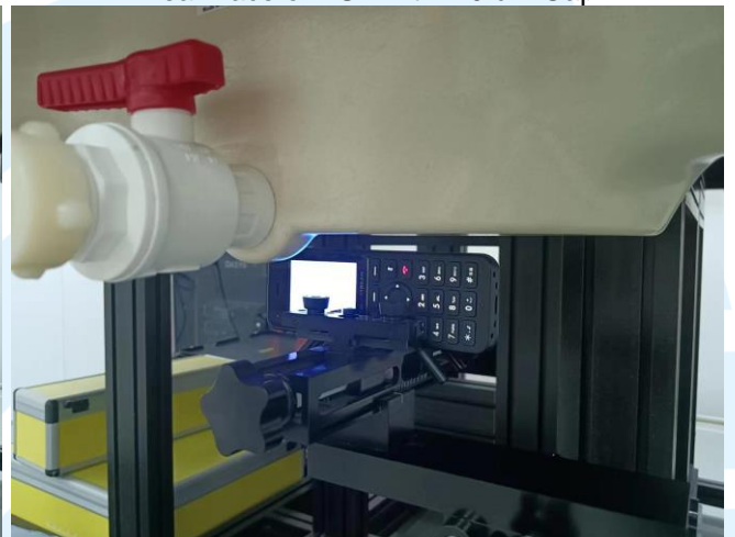
Right Side of EUT with 1.0 cm Gap
