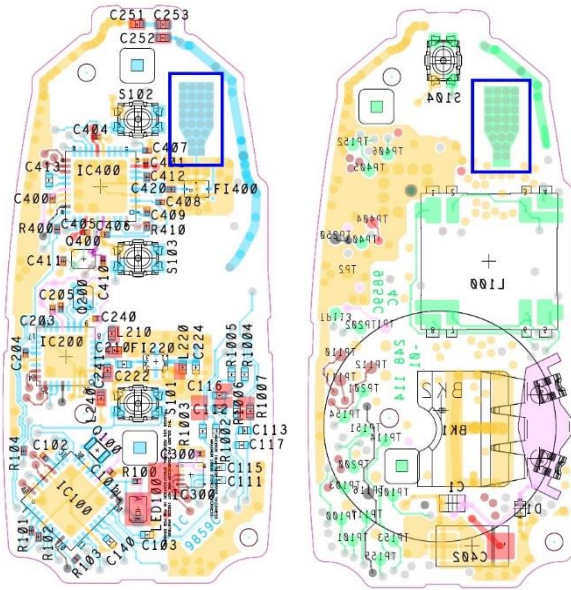
Picture 3: PCB integrated monopole UWB antenna
