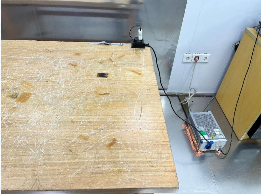
Photo of Setup for Radiated Emission (30MHz~1GHz)
