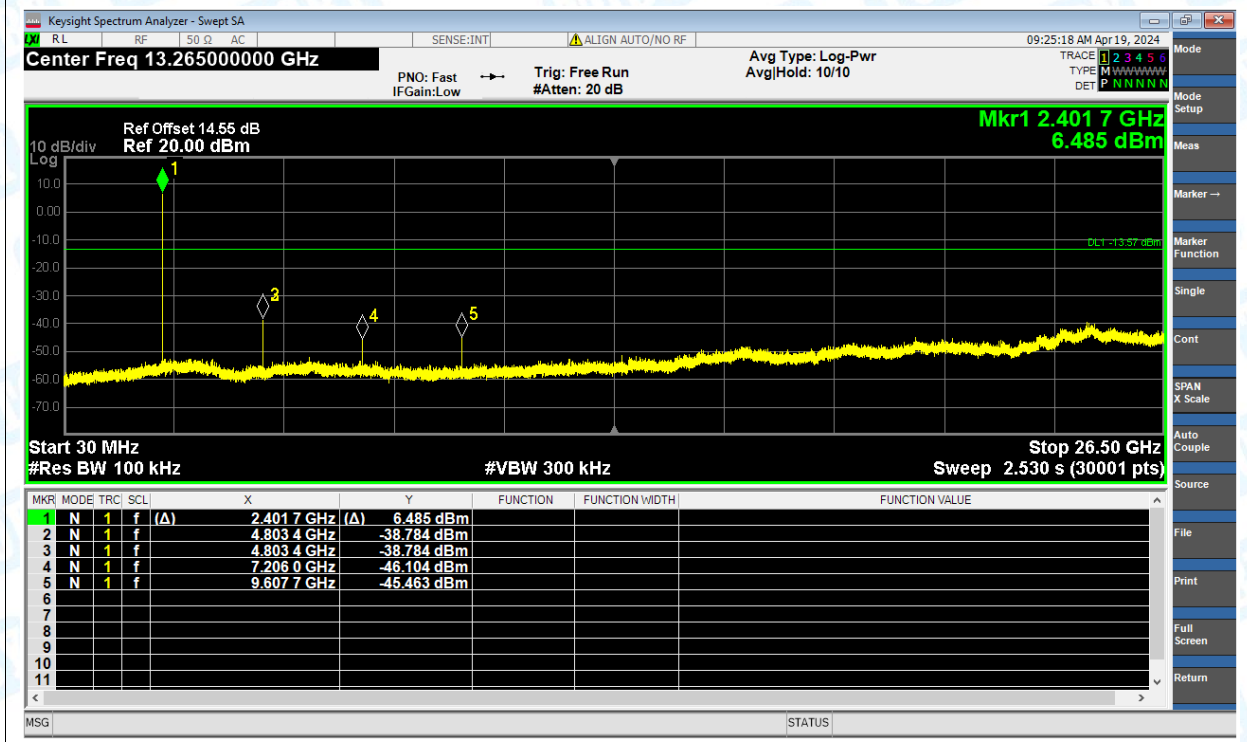
Tx. Spurious NVNT 1-DH1 2402MHz Ant1 Emission
