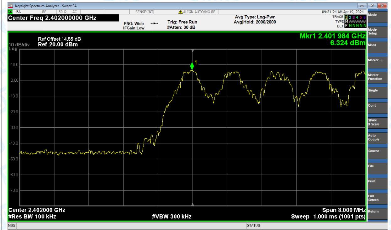
Band Edge(Hopping) NVNT 1-DH1 2402MHz Ant1 Hopping Emission
