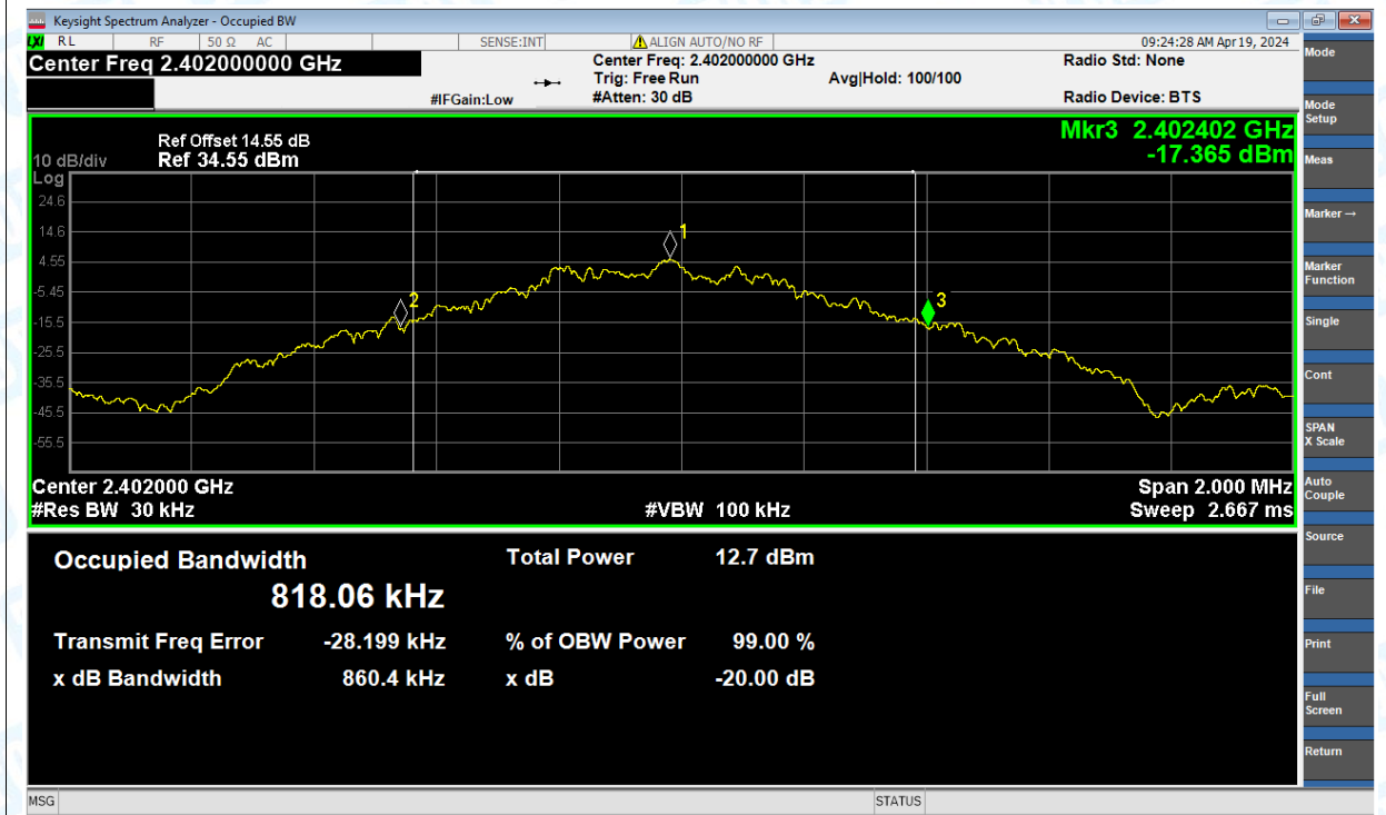
-20dB Bandwidth NVNT 1-DH1 2441MHz Ant1
