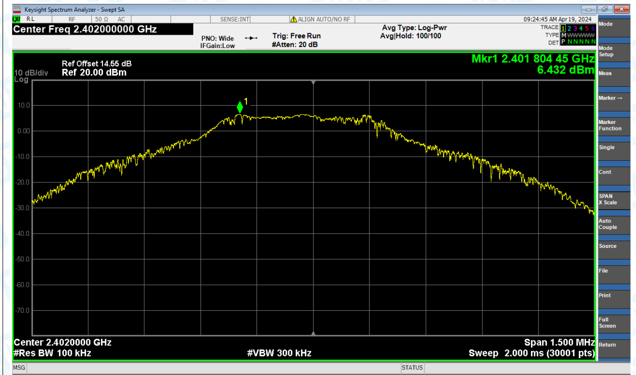
Tx. Spurious NVNT 1-DH1 2402MHz Ant1 Emission
