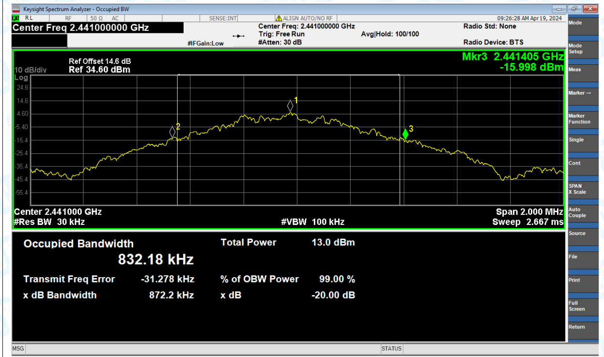
-20dB Bandwidth NVNT 1-DH1 2441MHz Ant1
