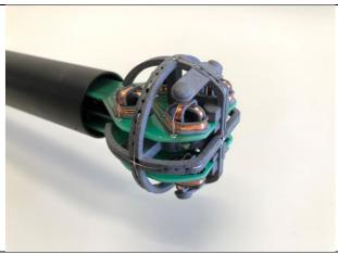
Test probe, without the casing
