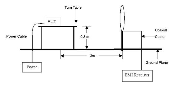
The diagram below shows the test setup that is utilized to make the measurements for emission from 30  $\,\mathrm{ll}$  to 1  $\,\mathrm{ll}$  emissions.
