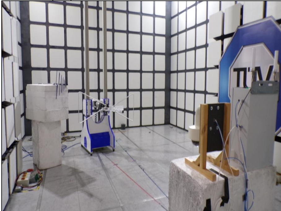
Figure 22 - Test Setup - 30 MHz to 1 GHz
