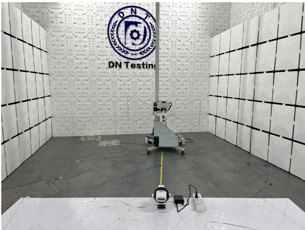
Radiated Emission Test View|(Below 1G)
