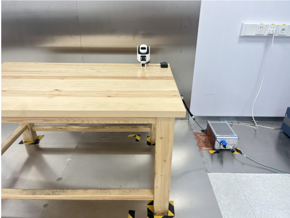
Radiated Emission Test View|(Below 1G)
