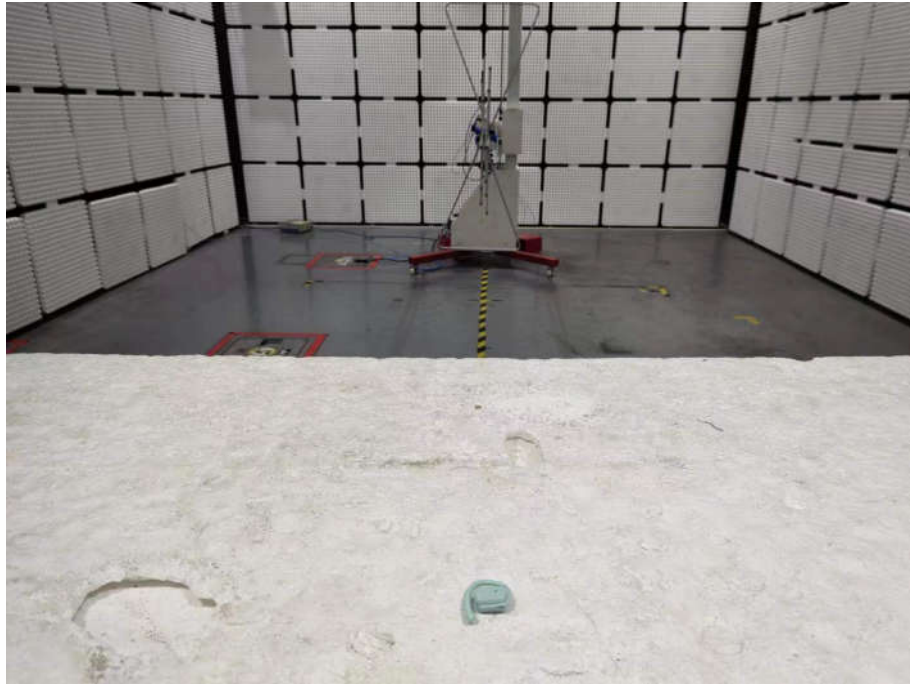
Radiated spurious emission Test Setup-3(Below 1GHz)(right ear)
