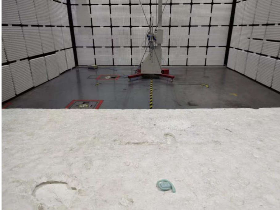
Radiated spurious emission Test Setup-1(Below 1GHz)(left ear)
