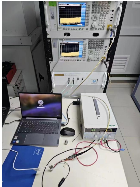
RF Conducted Test setup (BT/WIFI)
