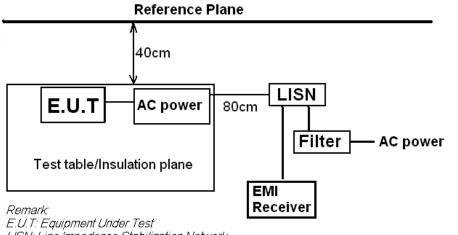
LISN: Line Impedence Stabilization Network
