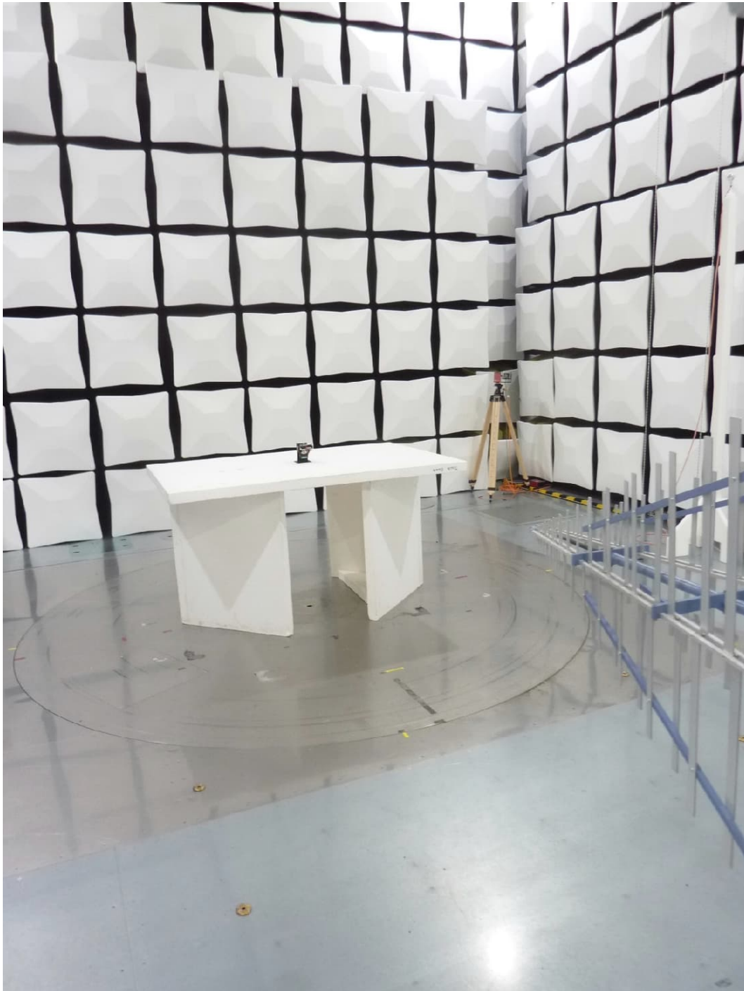
Test setup semi-anechoic chamber M276, 30 MHz – 1 GHz
