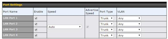
On this screen, you can enable specific ports, as well as determine the speed of the LAN ports, whether each port is a trunk or access port, can well as which VLAN each link belongs to, if any.
